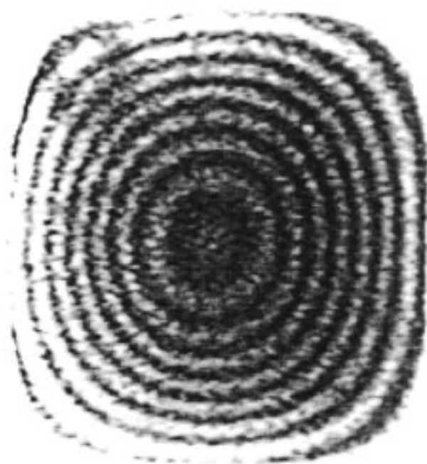
Figure 4. Holographic pattern (1,1 mode) for a membrane in anisotropic biaxial extension at 367 Hz.
